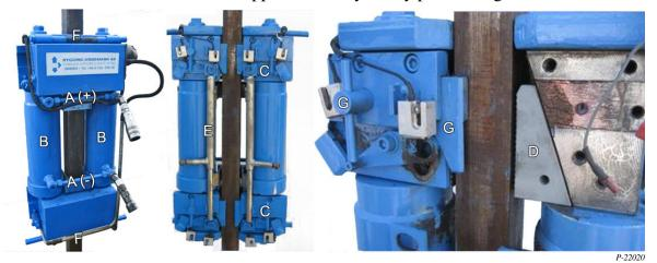
Fig. 1. (A) Branch pipe, (B) Hydraulic cylinders, (C) Grip jaw head, (D) Grip jaws, (E) Switch mechanism, (F) Top-bottom plate, (G) Catches with Operating shafts.
